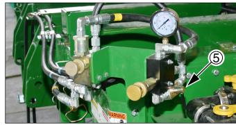
Figure 22 Lift-Assist Valve (Closed)
