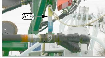
Figure 27 Applicator NH<sub>3</sub> Shut-Off Valve
